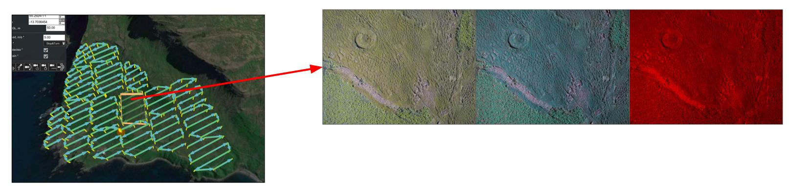
After images have been processed the photographs are merged together to create a single high-resolution image that is used as the base layer of the data infrastructure. Photogrammetry is applied to specific features such as buildings and known archaeological sites to create a layer of 3D models.
